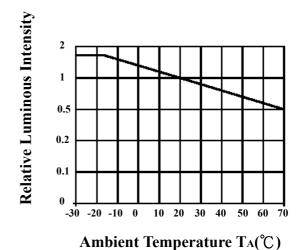
**Luminous Intensity Vs. Ambient Temperature**
